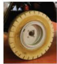
No-marking + foam filled tyres
