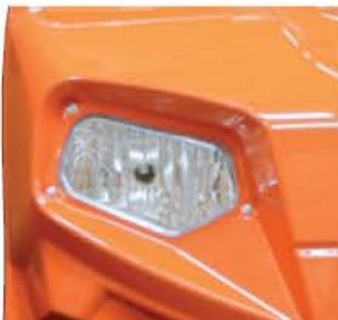
Low- and high-beam head lights
